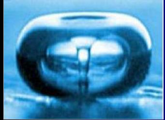
Imploding vapor bubble with jet (up to 100000 bar at the ground of the jet and temperatures of several thousand K !)
