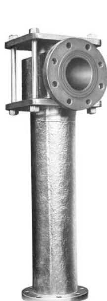
Fig. 12. Fig. 562 Steam Jet Ejector, constructed of impervious Graphite. Ejectors with 4" and above suction and pressure connections have fiberglass armoring. Nozzles are interchangeable with those used in the Fig. 555H Pump described on page 5.
