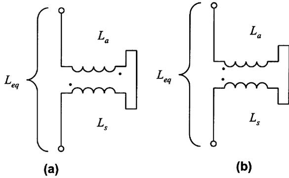
Fig. 2. The two electrical connections possible with helical gun geometry showing (a) additive magnetic fields and (b) subtractive magnetic fields.
