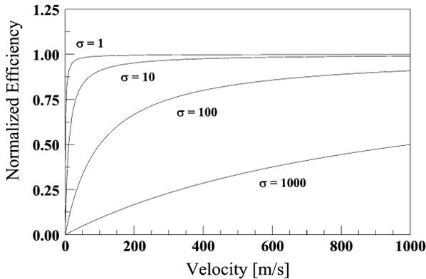
Fig. 3. Normalized efficiency versus velocity for various characteristic velocities.
