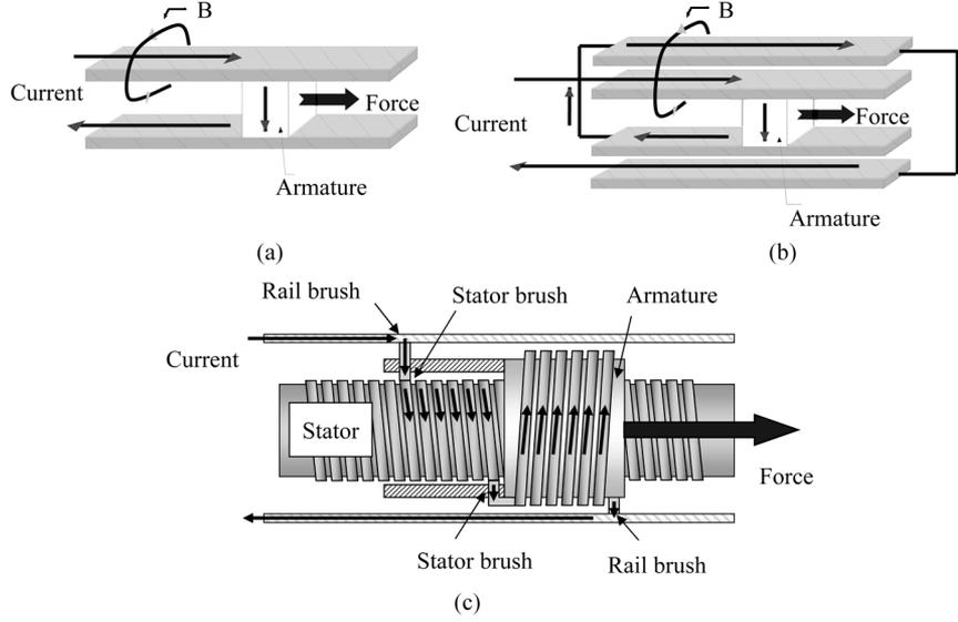
Fig. 1. Constant gradient EML geometry of the (a) conventional railgun, (b) augmented railgun, and (c) helical gun.
