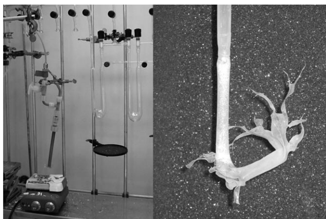
Figure 9. Typical damages caused by the explosions of about 0.5 mmol of N_5^+P(N_3)_6^- . In the left picture, the explosion destroyed the heavy ceramic plate of a stirring plate. The right picture shows the close-up of an exploded, originally straight Teflon reaction tube.
