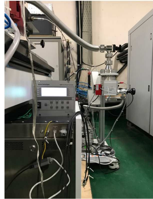
Vacuum pump with ion pump controller
