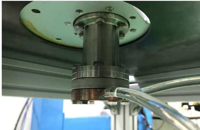
e-γ tungsten target for X-ray irradiation
