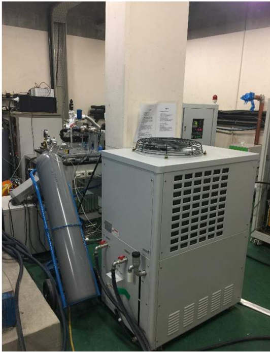
Cooling system with 0.1°C stability
