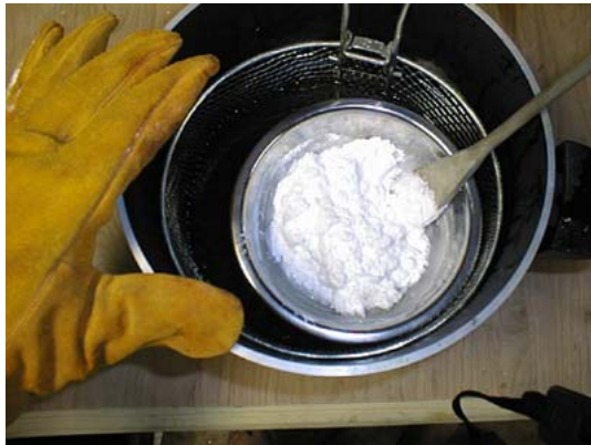
Figure 17: Left: Starting to melt the propellant mix. Right: Propellant ready for casting
