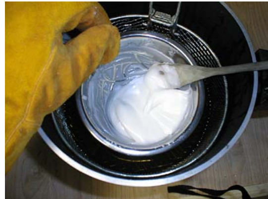
Figure 17: Left: Starting to melt the propellant mix. Right: Propellant ready for casting
