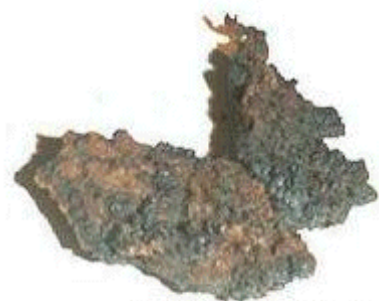
Charred remains of overheated propellant which failed to ignite
