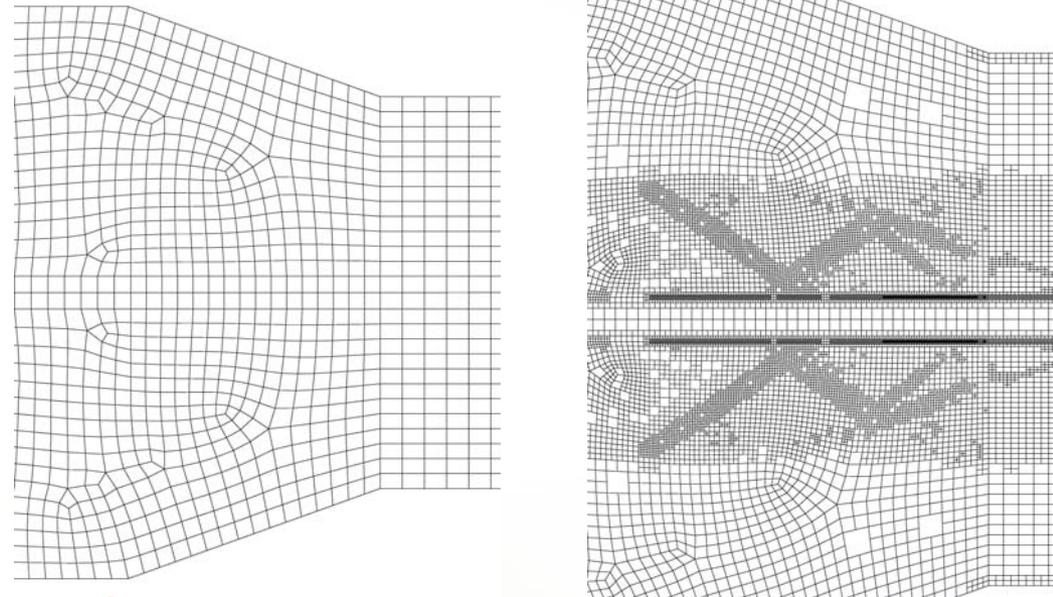
Adaptation following the pressure gradient, and  $y^+$  close to walls
