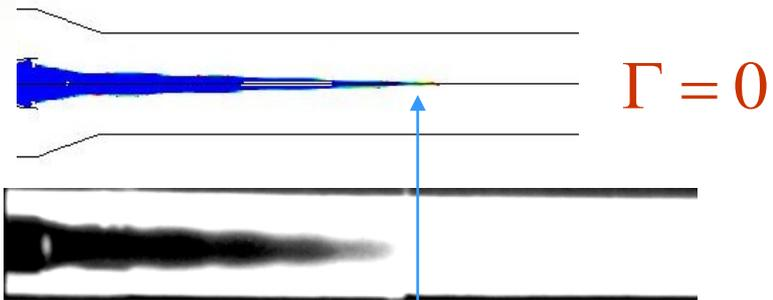
The laser tomography picture is treated by an image processing software to deduce  $l_m$  (Desevaux et al.)
