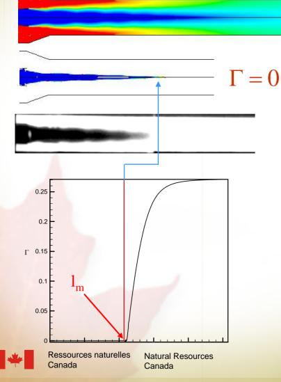
The laser tomography picture is treated by an image processing software to deduce  $l_m$ (Desevaux et al.)
